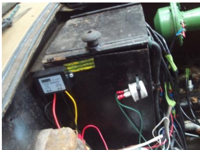
The little box is the converter. The pretty drum thing is the flasher unit. (see other article).
